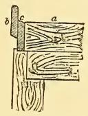
Fig. 20. Section through the cutting edge of table shown in Fig. 19.
