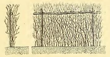
Fig. 11,-Diagram of fence intended to stop drift sand.
